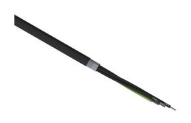
Helukabel TOPFLEX 600 VFD cable, shielded, 4 conductors (includes ground), 10 AWG, tinned copper, XLPE conductor insulation material, black with white numbers and green/yellow ground, PVC jacket, black, cut to length.
