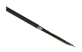
Helukabel TOPFLEX 600 VFD cable, shielded, 4 conductors (includes ground), 12 AWG, tinned copper, XLPE conductor insulation material, black with white numbers and green/yellow ground, PVC jacket, black, cut to length.
