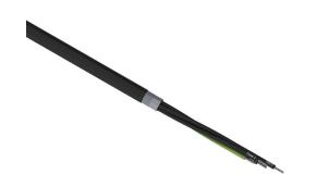
Helukabel TOPFLEX 600 VFD cable, shielded, 4 conductors (includes ground), 16 AWG, tinned copper, XLPE conductor insulation material, black with white numbers and green/yellow ground, PVC jacket, black, cut to length.
