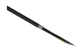
Helukabel TOPFLEX 600 VFD cable, shielded, 4 conductors (includes ground), 14 AWG, tinned copper, XLPE conductor insulation material, black with white numbers and green/yellow ground, PVC jacket, black, cut to length.
