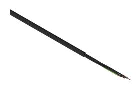
Helukabel TrayControl 600 flexible control cable, unshielded, 4 conductors (includes ground), 4 AWG, bare copper, PVC/Nylon conductor insulation material, black with white numbers and green/yellow ground, PVC jacket, black, cut to length.
