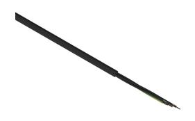
Helukabel TrayControl 600 flexible control cable, unshielded, 4 conductors (includes ground), 8 AWG, bare copper, PVC/Nylon conductor insulation material, black with white numbers and green/yellow ground, PVC jacket, black, cut to length.
