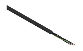
Helukabel TrayControl 600 flexible control cable, unshielded, 5 conductors (includes ground), 10 AWG, bare copper, PVC/Nylon conductor insulation material, black with white numbers and green/yellow ground, PVC jacket, black, cut to length.
