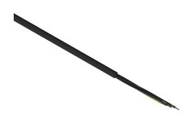
Helukabel TrayControl 600 flexible control cable, unshielded, 4 conductors (includes ground), 10 AWG, bare copper, PVC/Nylon conductor insulation material, black with white numbers and green/yellow ground, PVC jacket, black, cut to length.
