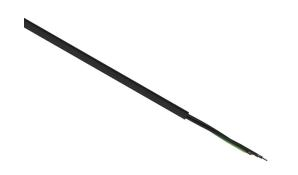
Helukabel TrayControl 600 flexible control cable, unshielded, 3 conductors (includes ground), 10 AWG, bare copper, PVC/Nylon conductor insulation material, black with white numbers and green/yellow ground, PVC jacket, black, cut to length.
