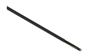
Helukabel TrayControl 600 flexible control cable, unshielded, 12 conductors (includes ground), 12 AWG, bare copper, PVC/Nylon conductor insulation material, black with white numbers and green/yellow ground, PVC jacket, black, cut to length.
