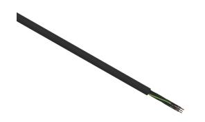
Helukabel TrayControl 600 flexible control cable, unshielded, 7 conductors (includes ground), 12 AWG, bare copper, PVC/Nylon conductor insulation material, black with white numbers and green/yellow ground, PVC jacket, black, cut to length.
