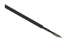
Helukabel TrayControl 600 flexible control cable, unshielded, 5 conductors (includes ground), 12 AWG, bare copper, PVC/Nylon conductor insulation material, black with white numbers and green/yellow ground, PVC jacket, black, cut to length.
