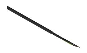
Helukabel TrayControl 600 flexible control cable, unshielded, 4 conductors (includes ground), 12 AWG, bare copper, PVC/Nylon conductor insulation material, black with white numbers and green/yellow ground, PVC jacket, black, cut to length.
