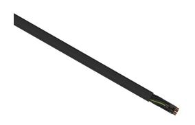
Helukabel TrayControl 600 flexible control cable, unshielded, 18 conductors (includes ground), 14 AWG, bare copper, PVC/Nylon conductor insulation material, black with white numbers and green/yellow ground, PVC jacket, black, cut to length.
