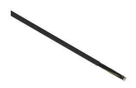
Helukabel TrayControl 600 flexible control cable, unshielded, 12 conductors (includes ground), 14 AWG, bare copper, PVC/Nylon conductor insulation material, black with white numbers and green/yellow ground, PVC jacket, black, cut to length.
