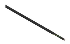
Helukabel TrayControl 600 flexible control cable, unshielded, 9 conductors (includes ground), 14 AWG, bare copper, PVC/Nylon conductor insulation material, black with white numbers and green/yellow ground, PVC jacket, black, cut to length.
