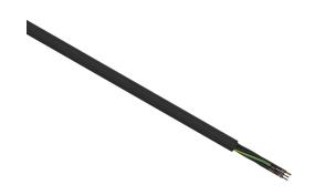
Helukabel TrayControl 600 flexible control cable, unshielded, 7 conductors (includes ground), 14 AWG, bare copper, PVC/Nylon conductor insulation material, black with white numbers and green/yellow ground, PVC jacket, black, cut to length.
