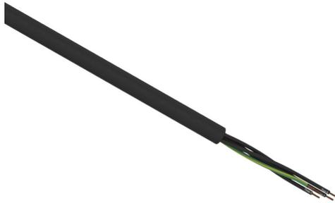
Helukabel TrayControl 600 flexible control cable, unshielded, 5 conductors (includes ground), 14 AWG, bare copper, PVC/Nylon conductor insulation material, black with white numbers and green/yellow ground, PVC jacket, black, cut to length.
