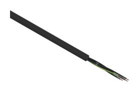
Helukabel TrayControl 600 flexible control cable, unshielded, 5 conductors (includes ground), 14 AWG, bare copper, PVC/Nylon conductor insulation material, black with white numbers and green/yellow ground, PVC jacket, black, cut to length.
