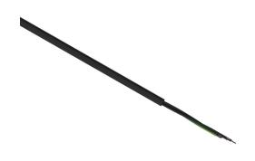
Helukabel TrayControl 600 flexible control cable, unshielded, 3 conductors (includes ground), 14 AWG, bare copper, PVC/Nylon conductor insulation material, black with white numbers and green/yellow ground, PVC jacket, black, cut to length.
