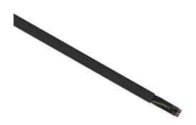
Helukabel TrayControl 600 flexible control cable, unshielded, 18 conductors (includes ground), 16 AWG, bare copper, PVC/Nylon conductor insulation material, black with white numbers and green/yellow ground, PVC jacket, black, cut to length.
