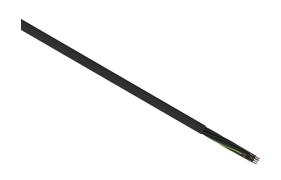
Helukabel TrayControl 600 flexible control cable, unshielded, 12 conductors (includes ground), 16 AWG, bare copper, PVC/Nylon conductor insulation material, black with white numbers and green/yellow ground, PVC jacket, black, cut to length.
