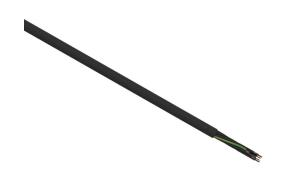
Helukabel TrayControl 600 flexible control cable, unshielded, 9 conductors (includes ground), 16 AWG, bare copper, PVC/Nylon conductor insulation material, black with white numbers and green/yellow ground, PVC jacket, black, cut to length.
