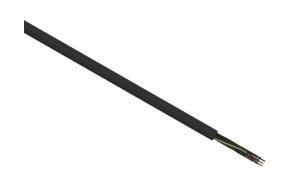
Helukabel TrayControl 600 flexible control cable, unshielded, 7 conductors (includes ground), 16 AWG, bare copper, PVC/Nylon conductor insulation material, black with white numbers and green/yellow ground, PVC jacket, black, cut to length.
