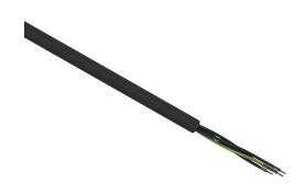
Helukabel TrayControl 600 flexible control cable, unshielded, 5 conductors (includes ground), 16 AWG, bare copper, PVC/Nylon conductor insulation material, black with white numbers and green/yellow ground, PVC jacket, black, cut to length.
