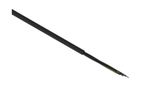
Helukabel TrayControl 600 flexible control cable, unshielded, 4 conductors (includes ground), 16 AWG, bare copper, PVC/Nylon conductor insulation material, black with white numbers and green/yellow ground, PVC jacket, black, cut to length.
