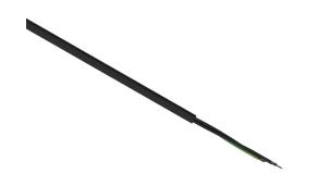
Helukabel TrayControl 600 flexible control cable, unshielded, 3 conductors (includes ground), 16 AWG, bare copper, PVC/Nylon conductor insulation material, black with white numbers and green/yellow ground, PVC jacket, black, cut to length.
