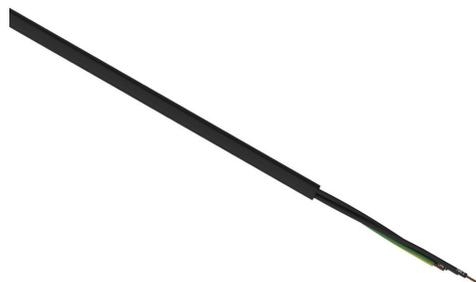
Helukabel TrayControl 600 flexible control cable, unshielded, 3 conductors (includes ground), 16 AWG, bare copper, PVC/Nylon conductor insulation material, black with white numbers and green/yellow ground, PVC jacket, black, cut to length.
