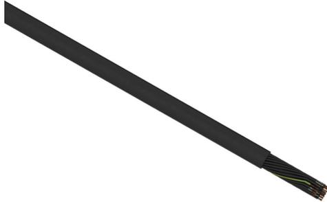
Helukabel TrayControl 600 flexible control cable, unshielded, 41 conductors (includes ground), 18 AWG, bare copper, PVC/ Nylon conductor insulation material, black with white numbers and green/yellow ground, PVC jacket, black, cut to length.
