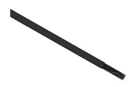
Helukabel TrayControl 600 flexible control cable, unshielded, 41 conductors (includes ground), 18 AWG, bare copper, PVC/Nylon conductor insulation material, black with white numbers and green/yellow ground, PVC jacket, black, cut to length.
