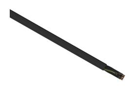
Helukabel TrayControl 600 flexible control cable, unshielded, 18 conductors (includes ground), 18 AWG, bare copper, PVC/Nylon conductor insulation material, black with white numbers and green/yellow ground, PVC jacket, black, cut to length.
