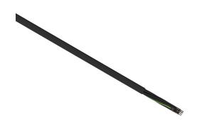
Helukabel TrayControl 600 flexible control cable, unshielded, 12 conductors (includes ground), 18 AWG, bare copper, PVC/Nylon conductor insulation material, black with white numbers and green/yellow ground, PVC jacket, black, cut to length.
