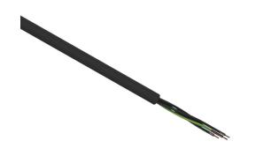
Helukabel TrayControl 600 flexible control cable, unshielded, 5 conductors (includes ground), 18 AWG, bare copper, PVC/Nylon conductor insulation material, black with white numbers and green/yellow ground, PVC jacket, black, cut to length.
