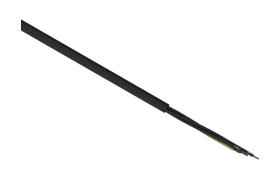
Helukabel TrayControl 600 flexible control cable, unshielded, 4 conductors (includes ground), 18 AWG, bare copper, PVC/Nylon conductor insulation material, black with white numbers and green/yellow ground, PVC jacket, black, cut to length.
