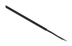
Helukabel TrayControl 600 flexible control cable, unshielded, 3 conductors (includes ground), 18 AWG, bare copper, PVC/Nylon conductor insulation material, black with white numbers and green/yellow ground, PVC jacket, black, cut to length.
