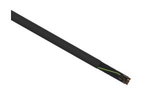
Helukabel TrayControl 600 flexible control cable, unshielded, 25 conductors (includes ground), 20 AWG, bare copper, PVC/ Nylon conductor insulation material, black with white numbers and green/yellow ground, PVC jacket, black, cut to length.
