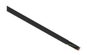
Helukabel TrayControl 600 flexible control cable, unshielded, 18 conductors (includes ground), 20 AWG, bare copper, PVC/Nylon conductor insulation material, black with white numbers and green/yellow ground, PVC jacket, black, cut to length.
