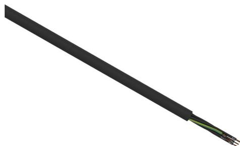
Helukabel TrayControl 600 flexible control cable, unshielded, 7 conductors (includes ground), 20 AWG, bare copper, PVC/Nylon conductor insulation material, black with white numbers and green/yellow ground, PVC jacket, black, cut to length.
