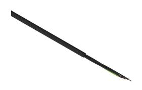
Helukabel TrayControl 600 flexible control cable, unshielded, 4 conductors (includes ground), 20 AWG, bare copper, PVC/Nylon conductor insulation material, black with white numbers and green/yellow ground, PVC jacket, black, cut to length.
