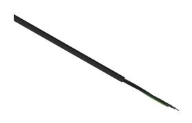
Helukabel TrayControl 600 flexible control cable, unshielded, 3 conductors (includes ground), 20 AWG, bare copper, PVC/Nylon conductor insulation material, black with white numbers and green/yellow ground, PVC jacket, black, cut to length.
