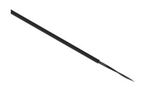
Helukabel TrayControl 600 flexible control cable, unshielded, 2 conductors, 20 AWG, bare copper, PVC/Nylon conductor insulation material, black with white numbers, PVC jacket, black, cut to length.
