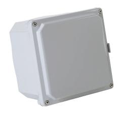
Integra Premium series enclosure, NEMA 1/2/3/3R/3S/4/4X/6/6P/12/13, 6 x 6 x 4in (HxWxD), wall mount, polycarbonate, light gray, gloss finish, screw cover.
