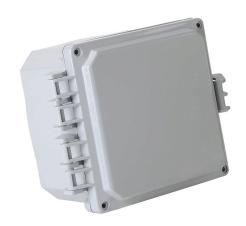
Integra Premium series enclosure, NEMA 1/2/3/3R/3S/4/4X/12/13, 6 x 6 x 4in (HxWxD), wall mount, polycarbonate, light gray, gloss finish, single-door, glass-filled nylon quick-release latch, padlock hasp and staple.
