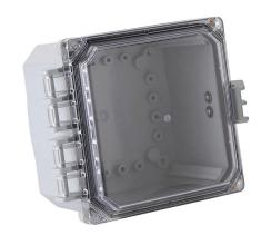
Integra Premium series enclosure, NEMA 1/2/3/3R/3S/4/4X/12/13, 6 x 6 x 4in (HxWxD), wall mount, polycarbonate, light gray, gloss finish, clear polycarbonate singledoor, glass-filled nylon quick-release latch, padlock hasp and staple.
