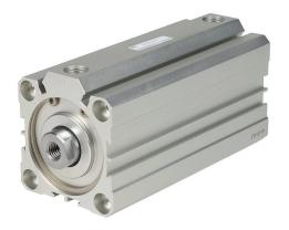
NITRA pneumatic cylinder, compact extruded, 50mm bore, 20mm rod diameter, 100mm stroke, double acting, magnetic piston, tapped end caps mount.
