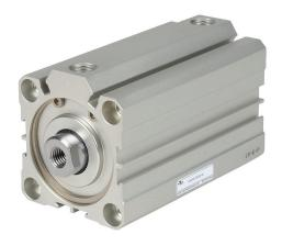
NITRA pneumatic cylinder, compact extruded, 50mm bore, 20mm rod diameter, 75mm stroke, double acting, magnetic piston, tapped end caps mount.
