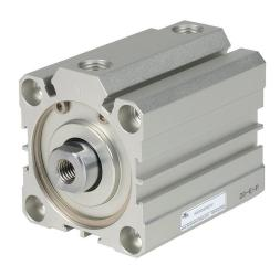
NITRA pneumatic cylinder, compact extruded, 50mm bore, 20mm rod diameter, 40mm stroke, double acting, magnetic piston, tapped end caps mount.
