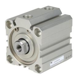
NITRA pneumatic cylinder, compact extruded, 50mm bore, 20mm rod diameter, 25mm stroke, double acting, magnetic piston, tapped end caps mount.
