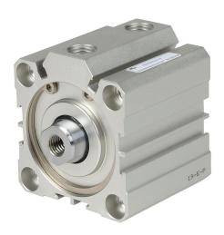
NITRA pneumatic cylinder, compact extruded, 50mm bore, 20mm rod diameter, 20mm stroke, double acting, magnetic piston, tapped end caps mount.
