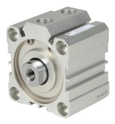
NITRA pneumatic cylinder, compact extruded, 50mm bore, 20mm rod diameter, 10mm stroke, double acting, magnetic piston, tapped end caps mount.
