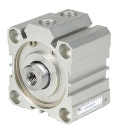
NITRA pneumatic cylinder, compact extruded, 50mm bore, 20mm rod diameter, 5mm stroke, double acting, magnetic piston, tapped end caps mount.
