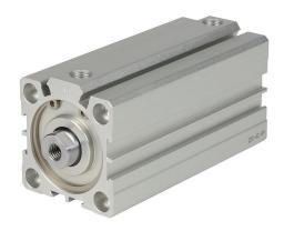
NITRA pneumatic cylinder, compact extruded, 40mm bore, 16mm rod diameter, 75mm stroke, double acting, magnetic piston, tapped end caps mount.
