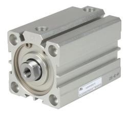
NITRA pneumatic cylinder, compact extruded, 40mm bore, 16mm rod diameter, 40mm stroke, double acting, magnetic piston, tapped end caps mount.
